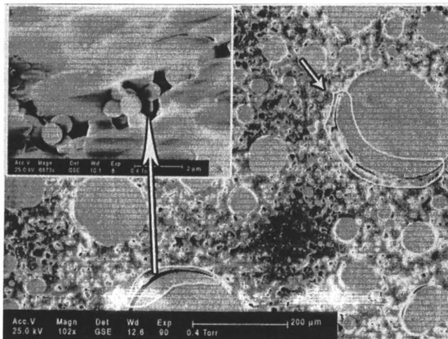
Figure 6e. SEM micrograph of surface morphology and surface detail of PC/PBrS (30/70).
